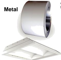
White Optics® Metal is available in coils up to 48" (1220mm) width and can be supplied as custom slit coils or cut-to-length sheets. It is supplied with a remov-able protective film and can be formed in most metal forming processes including punching, press brake and die forming.
