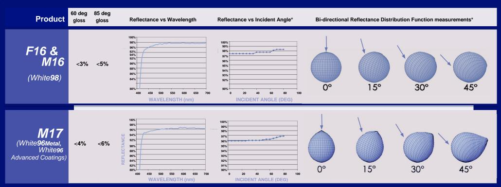
\*Reflectance and BRDF testing performed by LTI Optics and available in Photopia modeling software
